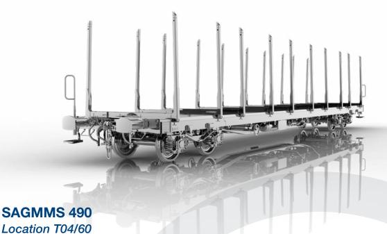
6-axle flat freight railway wagon with 101 t bearing capacity ranks among versatile wagons, which are used for transportation of ISO containers (20' and 40') and swap bodies, heavy tracked and wheeled military vehicles and heavy industrial cargo (steel semi-finished products, rolled profiles, rails, bars, pipes, plates, etc.).
